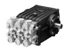
T Series 47, Triplex Plunger Pump, Solid Shaft – Forged brass manifold with an exclusive lifetime warranty. Heavy duty tapered roller bearings and over sized connecting rods for maximum life.
